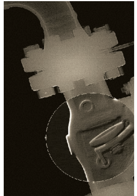
Computed Radiographic image of a valve and valve seat, showing the advantages of the wide dynamic range of the imaging plate. In this example the valve seat area has been selected for further analysis.
