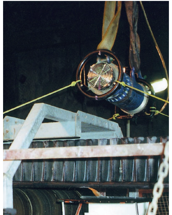
Fluoroscopic inspection setup
