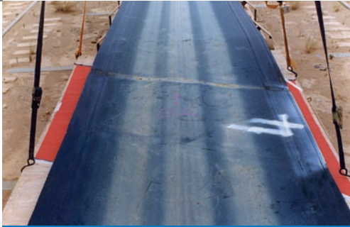
Radiographic film positioned under conveyor belt
