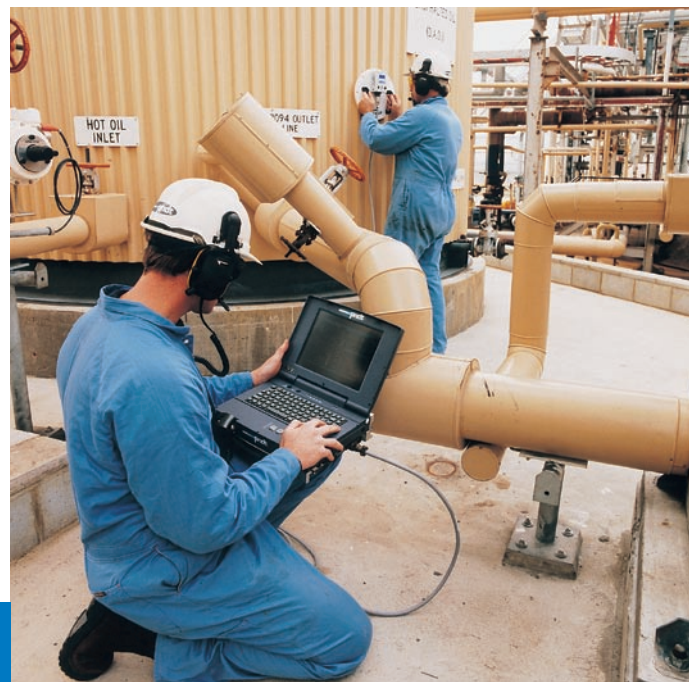
Incotest being carried out on an insulated storage tank
